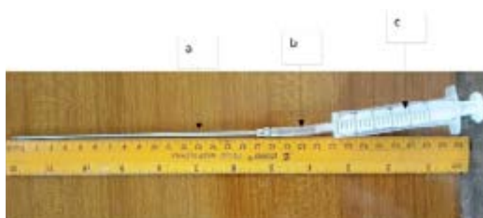
Figure 1: Aspirating long needle of an automatic syringe attached to ingress tube and syringe a: aspirating long needle; b: ingress tube; c: syringe
